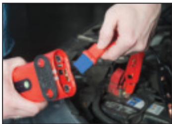
Once it Starts, Disconnect Clamps from Weego 66
