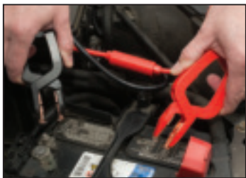
Detach Clamps From Battery
